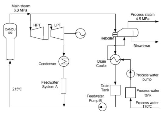
Fig. 1. Typical large nuclear unit secondary side configuration.
